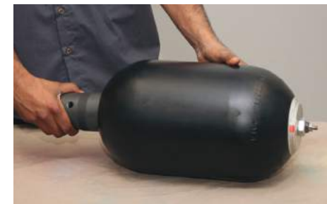
7) Slide the Anti extrusion ring on the port body. Pull the port out until the Anti-extrusion ring is seated into the shell opening.
