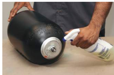
14) Follow the instructions and fill the accumulator with desired nitrogen precharge pressure at a slow rate. Using soap water check the gas valve for any leaks. Tighten the core or the gas valve to stop the leak. Replace the core or the gas valve is necessary.
