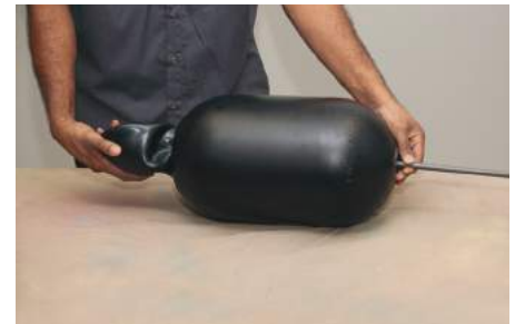
4) Lubricate the bladder with the system fluid. Attach a bladder pull rod to the gas valve shroud thread and pull the bladder gently into the shell.
