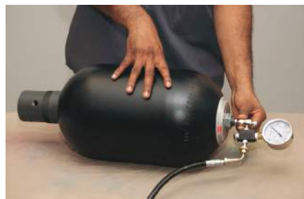
8) Using the charging assembly, fill slowly nitrogen pressure up to 25 psi (1.7 bar) to properly position the port and the anti-extrusion into the opening.
