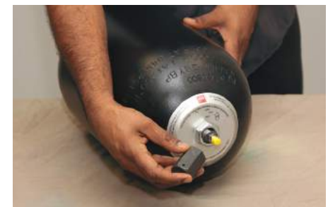
16) Replace the protective cap and hand tighten. Tighten the lock nut and the jam nut.
