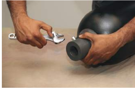
12) Install the bleeder plug and tighten it with the wrench.
