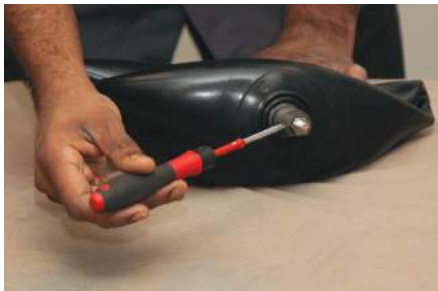
3) For smaller size bladders when there is no gas valve present, install the valve core using the valve core tools and torque it to 4 In-Lbs (0.45 Nm).
