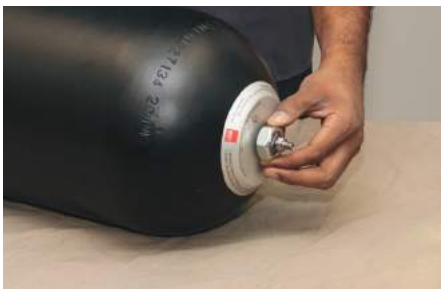
5) Install the Name plate and jam nut on to the valve stem. Hand tighten the jam nut.
