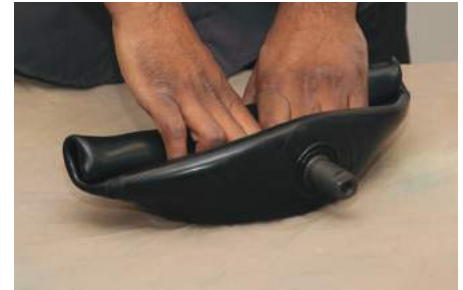
1) Squeeze the bladder as shown to release any air trapped inside the bladder.
