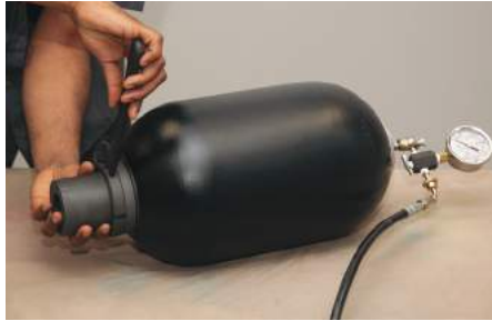
11) Install the spacer and locknut. Tighten the locknut using the spanner wrench.
