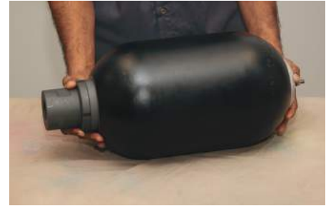
13) Turn the shell around its axis to allow uniform lubrication of the bladder.
