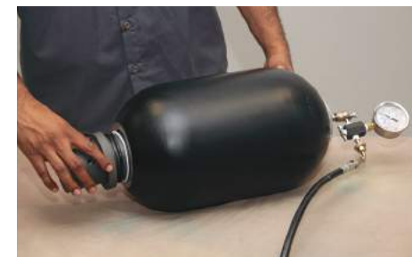
10) Install the Teflon back up followed by the O-ring and rubber back-up.
