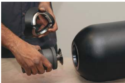
6) Insert the fluid port body followed by the Anti-extrusion ring into the shell.
