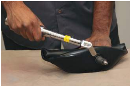
2) Install the gas valve adaptor into the valve stem. Torque it to 90 In-Lbs(10 Nm).
