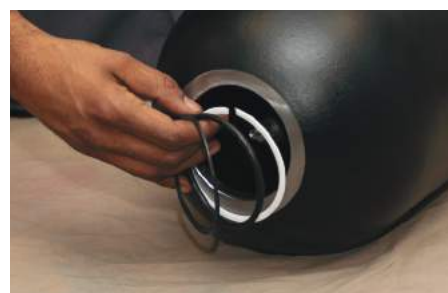
9) Remove the O-Ring back up, O-Ring & Teflon rings.
