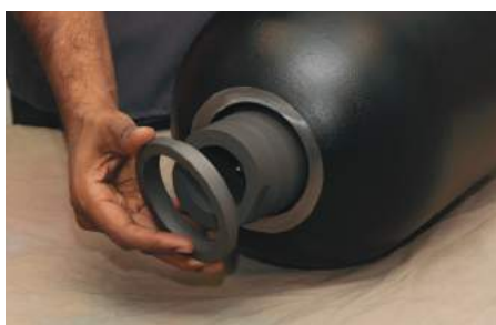
7) Remove spacer ring. For the next steps, care should be taken not to drop parts inside the shell if the service is conducted while the accumulator is vertical installed in the system.
