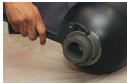
6) Remove the locknut using the spanner wrench.
