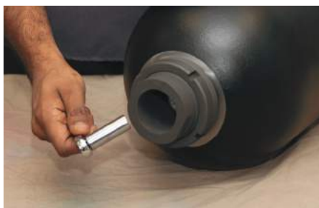
4) Remove the gas valve adaptor using an appropriate socket wrench. Skip this step if the accumulator is mounted vertical on system.
