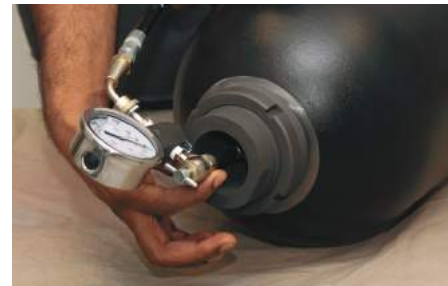
3) Discharge completely the nitrogen precharge pressure using the charging & gauging assembly.
