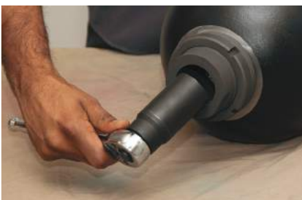
5) Remove the Jam nut using appropriate socket wrench.
