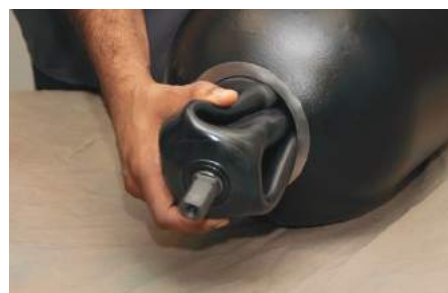
12) Remove the bladder from the shell by squeezing out any residual gas in the bladder.
