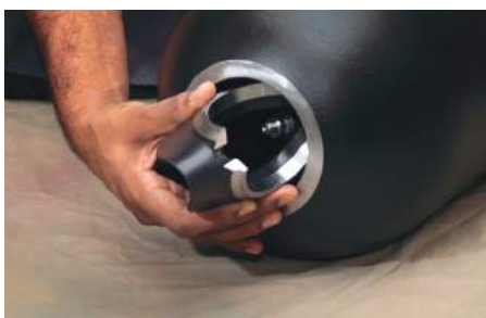
10) Remove the Anti-Extrusion ring from the top adaptor. Fold the ring and retrieve from the shell.
