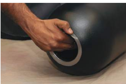
8) Push the top adaptor inside the shell. If it does not go inside possibly due to trapped residual pressure, consult factory.
